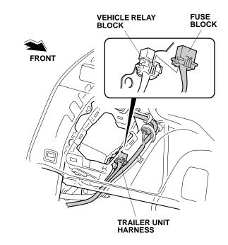
24. Secure the trailer unit harness to the vehicle harness with three wire ties.
