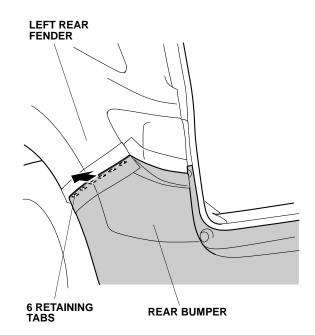
• Release one retaining tab on each side of the bumper.
