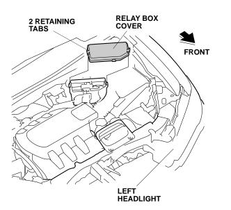
37. Plug the 20A fuse into the relay box as shown.
