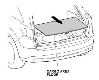
3. Remove the cargo area front floor lid (four clips).
