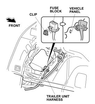
22. Secure the fuse block on the trailer unit harness to the vehicle panel. Go to step 24.
