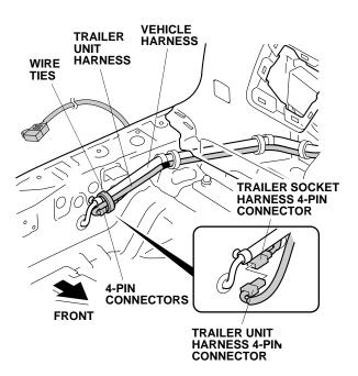
31. Align the green tape on the trailer socket harness to the vehicle clip, and secure the trailer socket harness to the vehicle harness with a wire tie.
