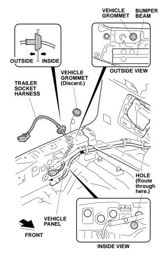
29. Route the trailer socket harness through the vehicle panel as shown, and secure the grommet on the trailer socket harness to the vehicle panel.
