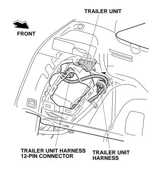
19. Secure the trailer unit harness to the vehicle harness with two wire ties.
