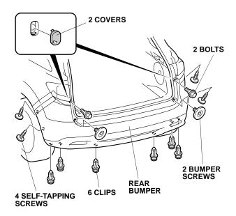
• Release six retaining tabs on each side of the bumper.
